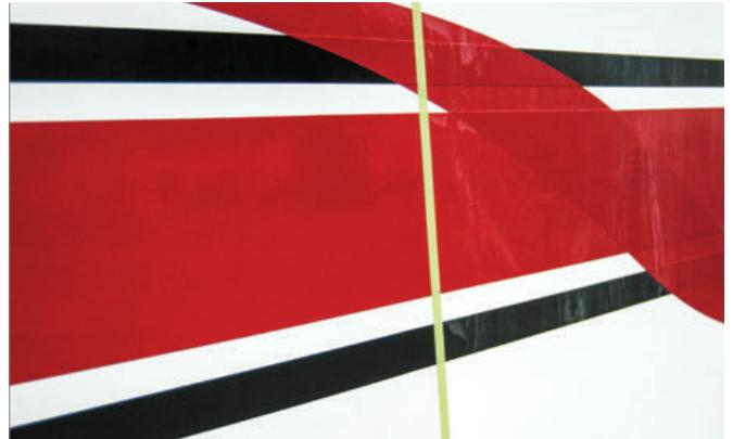
Scrubbing the RV's exterior fiberglass and striping with Poli Prep and applying five coats of Poli Glow sealer removed the stains (right of green tape) and brought back the shine (left of green tape). The Poli Glow process is safe for decals and graphic elements.
